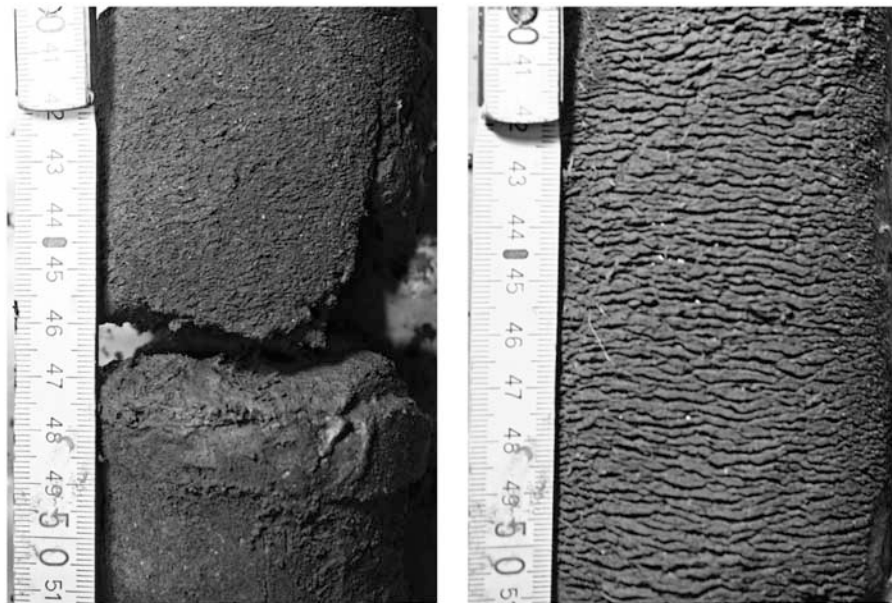
Figure 3. Core samples obtained from the intercircle area (left photo) and circle (right photo) at the Franklin Bluffs site during winter. On the right photograph, a sequence of horizontally oriented ice lenses can be observed. The vertical scale is in centimeters.
