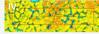
(IV.) The imagery and microrelief layer were stacked and input along with the training samples to train a random forest classifier [5]. The classified output was generalized to remove small, noisy patches of units.
