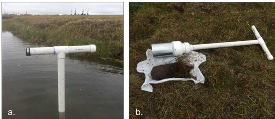
*Figure 3.* Photos of coring device used to collect biomass and soil samples, showing (a.) corer inserted into pond sediment with cap sealing the open handle, and (b.) intact core sample removed from the device post-extraction. Photos by EWC.
