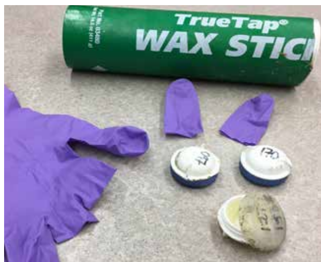
Figure 2.7. Tube wax, rubber gloves and contact lens cases purchased at the Prudhoe Bay General Store were used to keep temperature loggers drier in the field. Failure rates were lowest when iButtons were coated in the soft wax before being placed in the cut off finger of a Nitrile rubber glove, which was then knotted and placed in a small plastic bag. Photo: IMG 5519.
