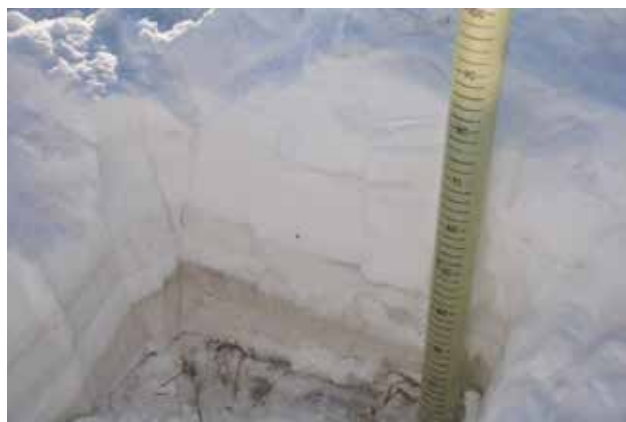
Figure 3.6. Snow pit at plot T2-005-T (Colleen Site A, Transect 2, 5 meters from road, polygon trough). Note the overall deep snow (97 cm), brown layers of dirty snow caused by road dust, several layers of high-density wind-packed snow, a thin hard layer at 8–19 cm (probably caused by a rain-on-snow event), and the dirty depth-hoar layer at the base of the snowpack. See profile in Appendix B. Photo: DSC 8811.
