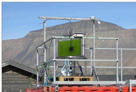
Fig. 1. Medium-scale (20L) photobioreactor in CARS USB in Longyearbyen, Svalbard.
