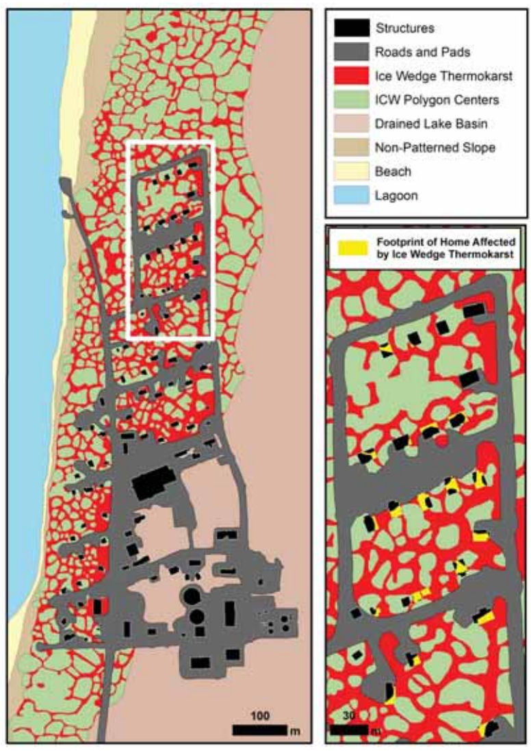
Generalized terrain units and infrastructure in Point Lay were mapped from an orthophoto mosaic and digital terrain model based on drone imagery. Estimates of the footprint of homes impacted by ice wedge thermokarst are shown in yellow in the inset map at lower right and in the histogram at top right.
